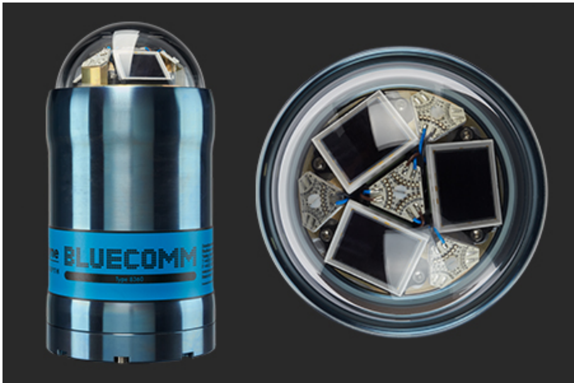
Figure 30 Bluecomm, wireless optical communication trough seawater
