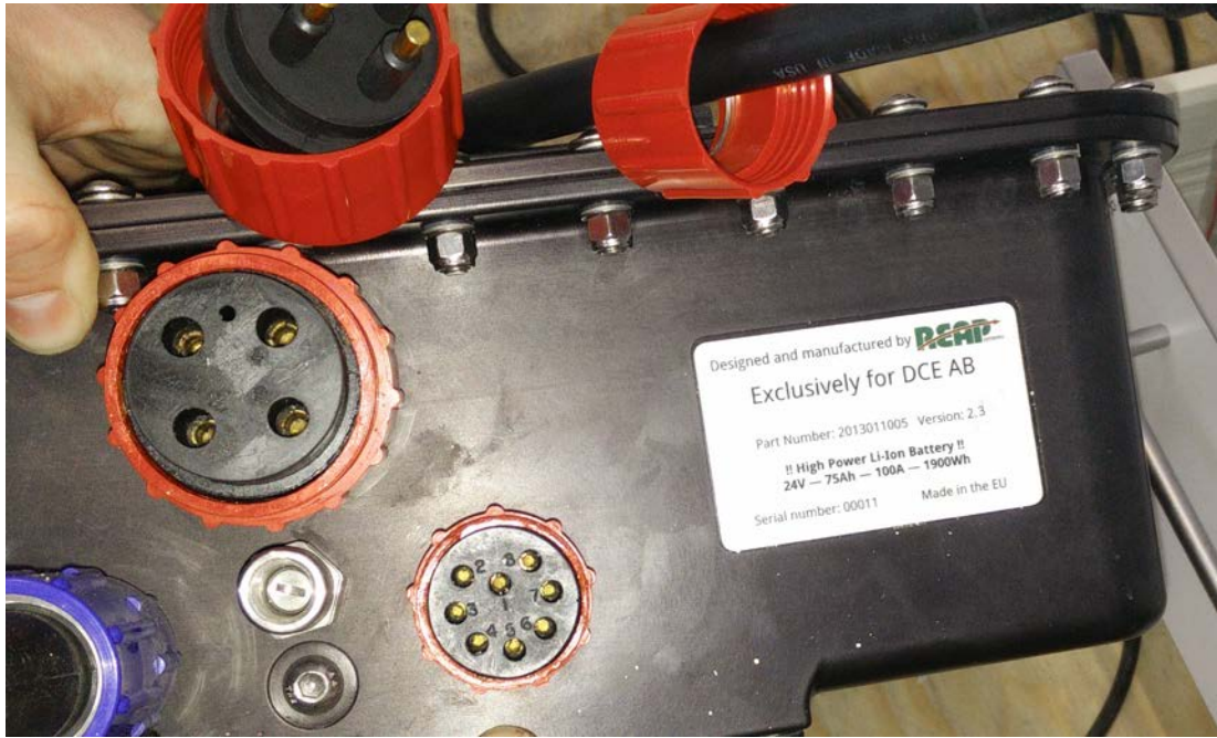
Figure 25 Reap Li-Ion 1900Wh, size 500x400x150mm
