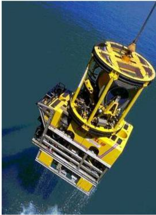
Figure 5 ROV attached to TMS during recovery (CQI, 2008)
