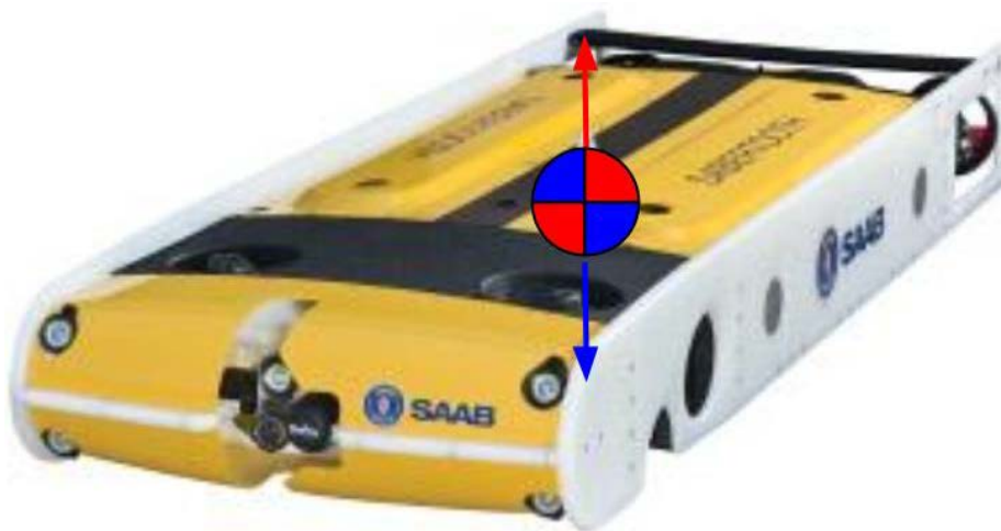
Figure 35 Center of mass and buoyancy are in the same position the center for an active stabilized vehicle
