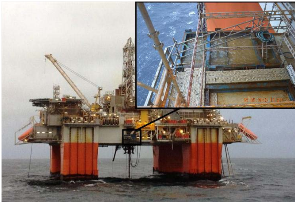
Figure 39 Location of the Rigs A-frame and winch system, Picture taken on student field trip for Statoil
