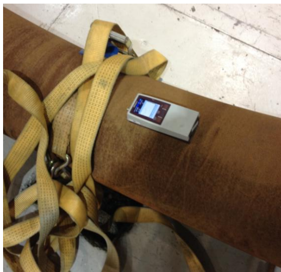
Figur 5-5: Ruhetsmåler under testing (MSS).
