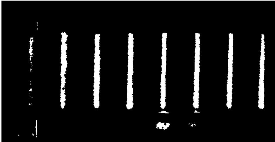
Figure 4.4: False positive object detection on the conveyor belt due to illumination. The figure shows the difference between the (i-1) -th and i -th frame as an binary image.
