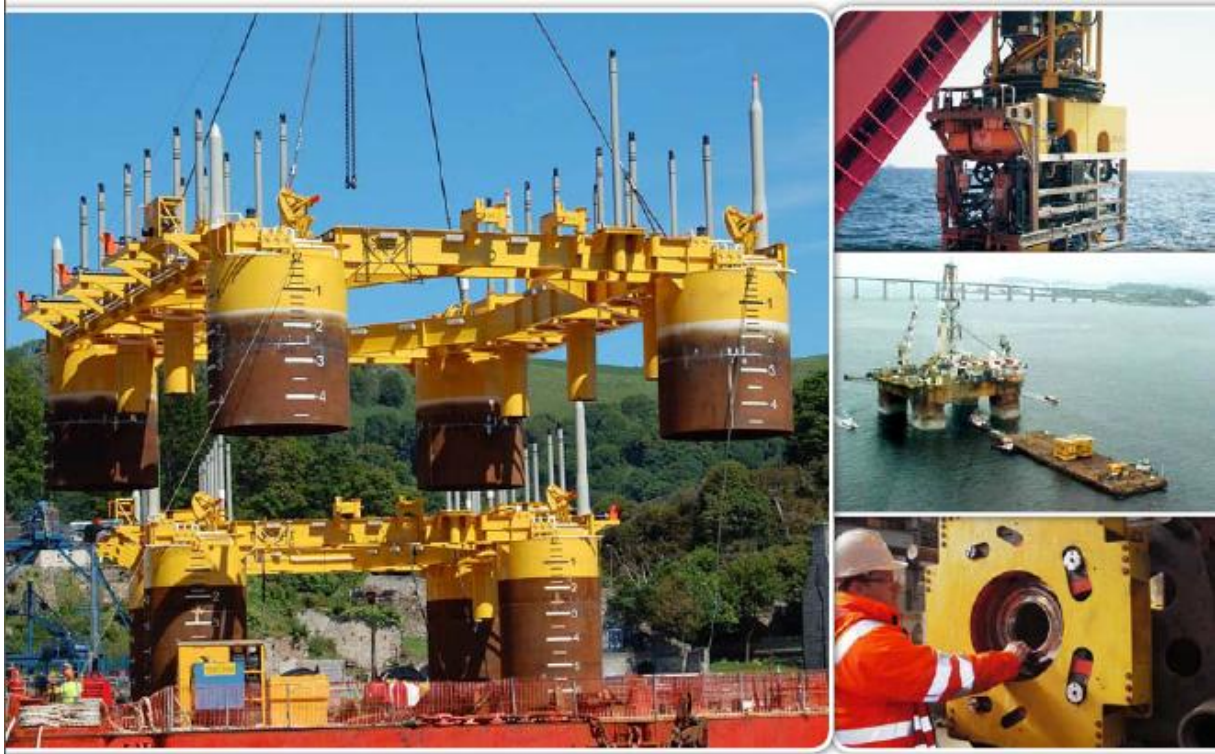
Figure 32 Subsea manifold and connection systems (GE oil and gas, 2011)
