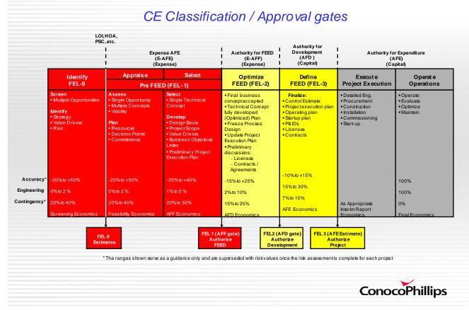
Figure nr.6: Requirements for estimation, (CPMS Cost Estimating Standard, 2007)
