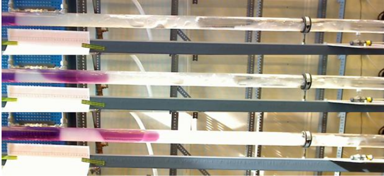
Figure 28: Gel plug run with remains of gel in front
