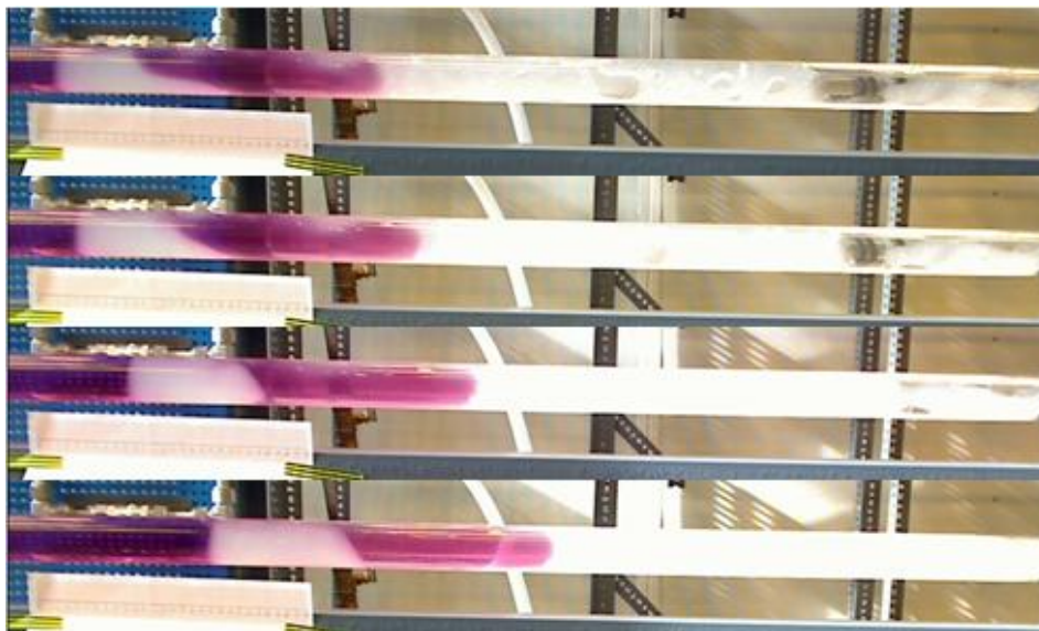
Figure 32: Moving of gel plug which has been split and settled for 2 hours
