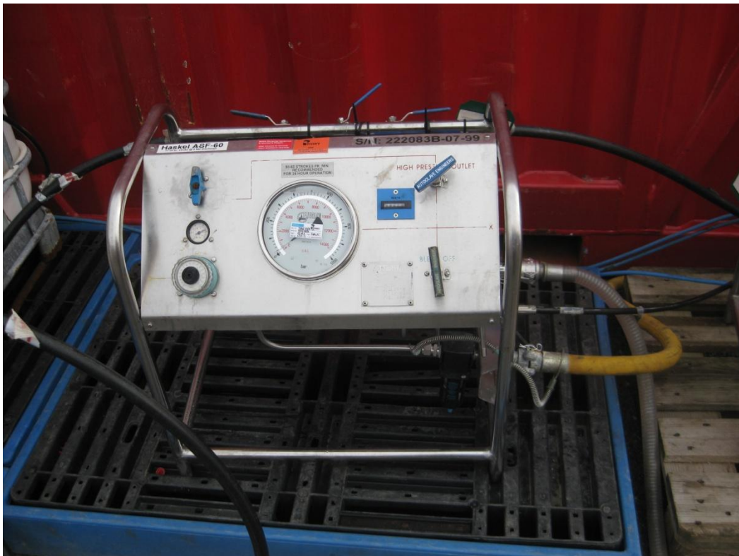
Appendix 8: Chemical injection pump
