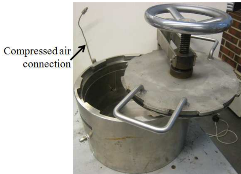
Figure 3.3: The aging cell, with connection for compressed air, used for aging of chalk cores prior to testing.
