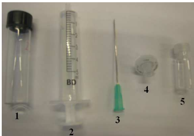
Figure 3.15: The equipment for filtering diluted samples prior to chemical testing. 1: Sample glass of diluted effluent water. 2: Syringe. 3: Needle. 4: Filter. 5: IC glass.
