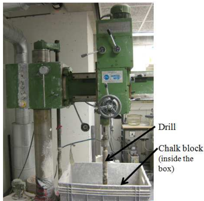
Figure 3.17: The drilling machine.
