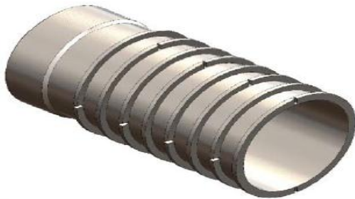
Figure 19: The hybrid ICD design uses a distributive geometry (Garcia et al. 2009).
