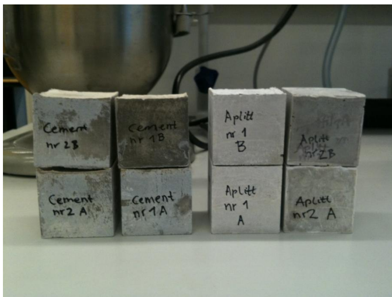
Figure 18 - The picture shows the samples 24 hours after setting and before the cubes were exposed to water.
