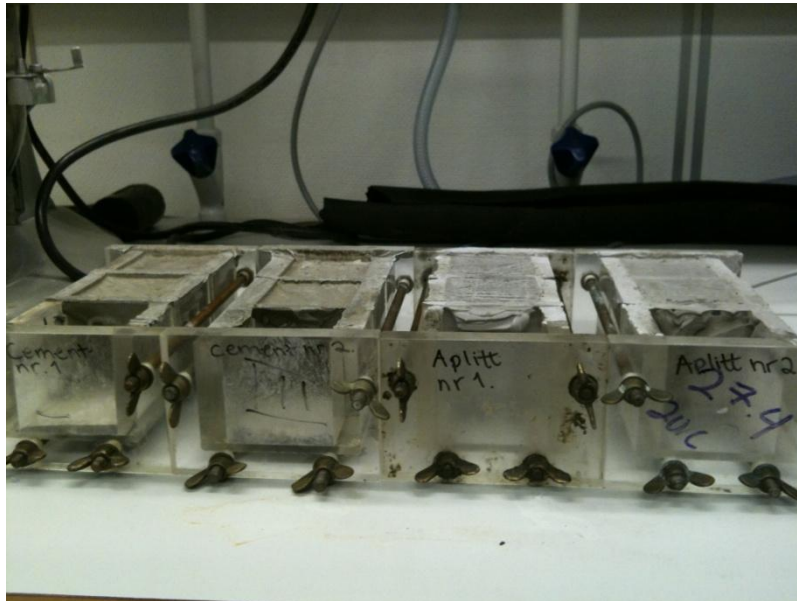
Figure 17 - Result of the shrinking test for Aplite and G cement. More detailed data can be found in Appendix A and B.
