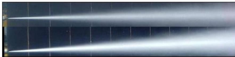
Figure 51 - The abrasive water jets leaving the nozzles [57].
