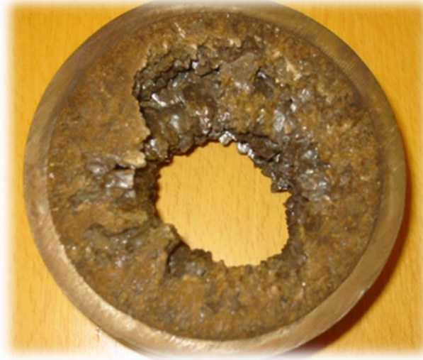
Figure 2-7 Calcium sulfate in a production tubing
