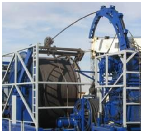
Figure 3-3 Coiled tubing on a reel [24].
