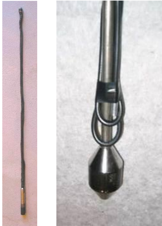
Figure 3-6 String shots and a detonating cord taped to a steel bar [27]
