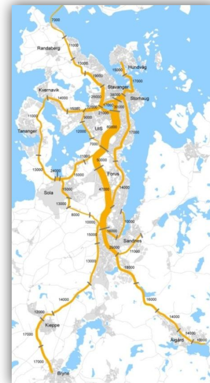
To the left: Figure 4.2.4 ÅDT illustration of traffic volume in the region. Source KVV
