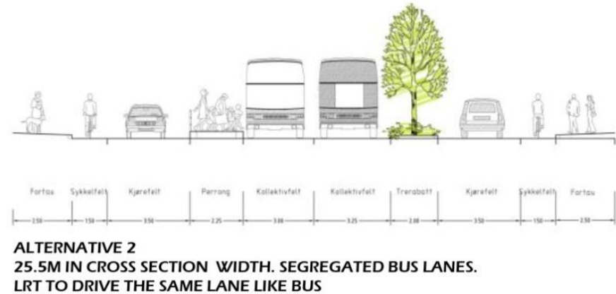
Figure 5.0.3 Alternative 2 cross section shows the four different zones of mobility. Figure 5.0.4 Alternative 2 cross section shows the boarding process
