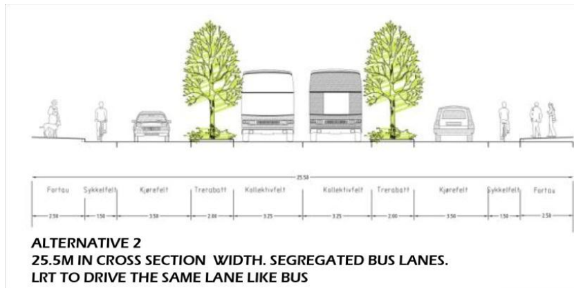
Figure 5.0.3 Alternative 2 cross section shows the four different zones of mobility. Figure 5.0.4 Alternative 2 cross section shows the boarding process
