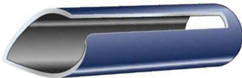
Figure 4-12- Orientating groove inside SPM [41]
