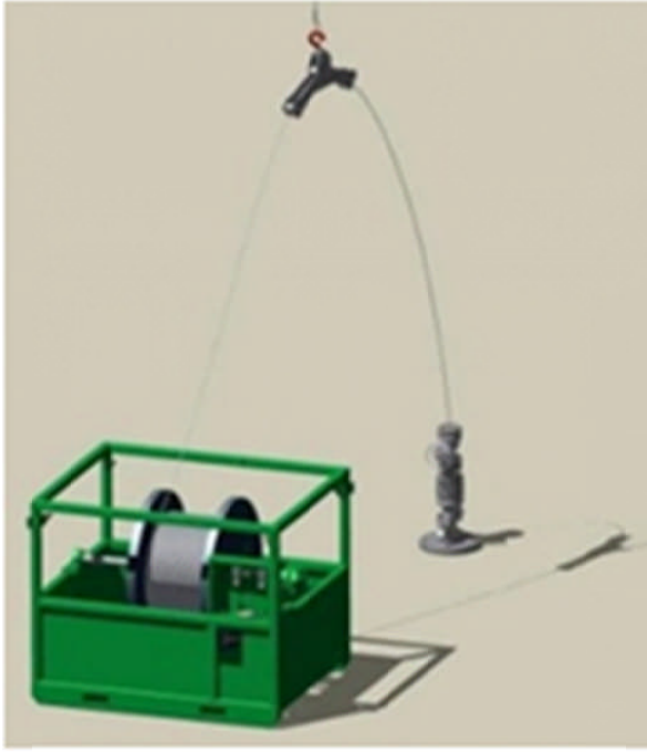
Figure 4-46- Illustrates control line installation [52]
