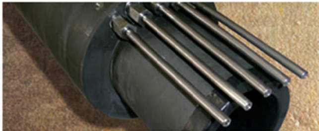
Figure 4-27- Production packer with control line feed through [48]
