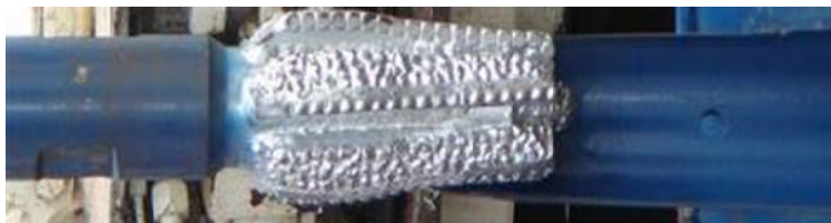
Figure 2-13- Casing mill for whipstock [21]
