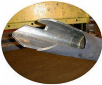
Figure 5-6- Orienting profile in liner hanger packer [23]
