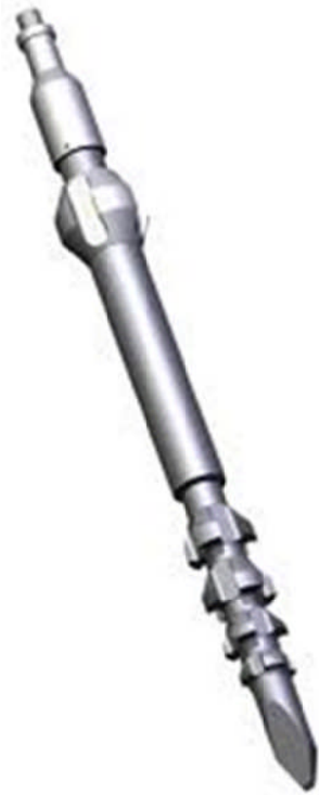
Figure 8-10- Spear for breaking glass plug [62]
