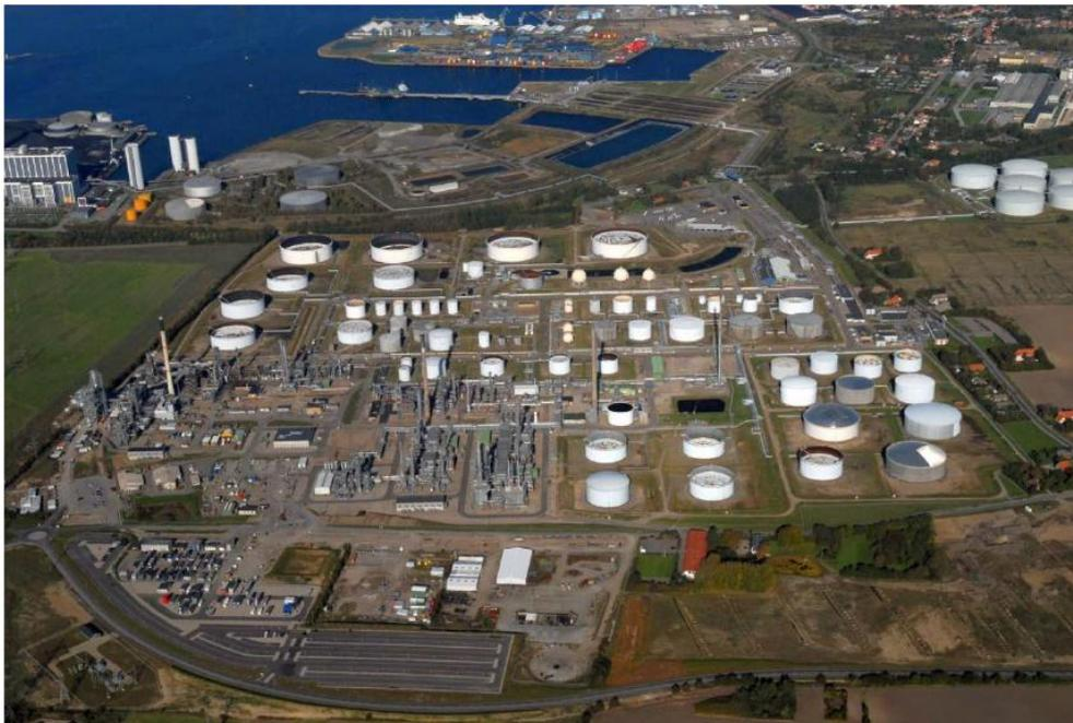
Figure 3.3: Picture of the Kalundborg refinery. The process area is in the lower left corner of the plant. The dock is in the upper part of the picture. The six tanks just visible in the far right of the picture belong to Foreningen Danske Olieberedskapslagre (FDO), but are operated by Kalundborg refinery[15]
