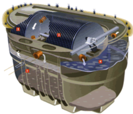
Fig.1.3.1. RBC unit for 25-70 pes (From http://www.wee-engineer.com/biodisc.htm )
