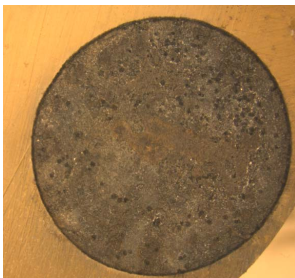
Figure 16. Picture of the working electrode for the experiment with a concentration of sulfide 50mM.
