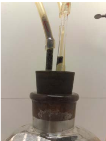
Picture Nr. 15: Water vapour on the top of bioreactor (internally)
