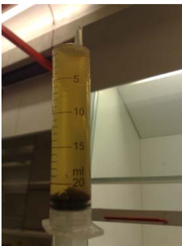
Picture Nr. 27: Industrial wastewater sample (Sleipner) with high content of methanol and MEG, from Karstø plant
