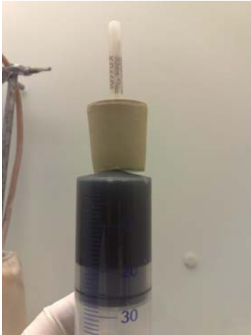
Picture Nr. 20: "Microsystem installed" (syringe with sample of bioreactor and 5 g/L of sugar concentration). No bubbles of air were left inside.
