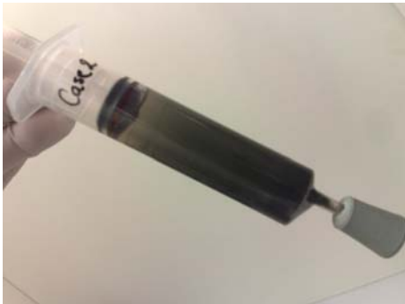
Picture Nr. 30: 1 week after installation of 4 syringes as “microsystem”. This is Case Nr. 2 (4mL Sleipner sample + 15 mL of Bioreactor sample+ 1mL wastewater as nutrient source)
