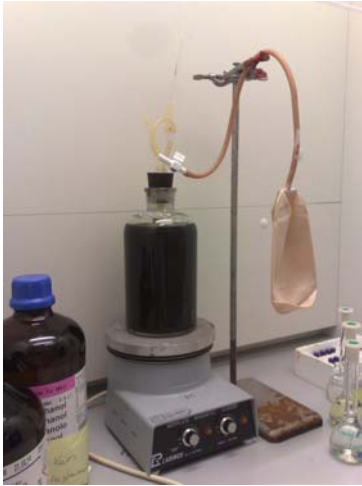
Picture Nr. 9: Installation of bioreactor
