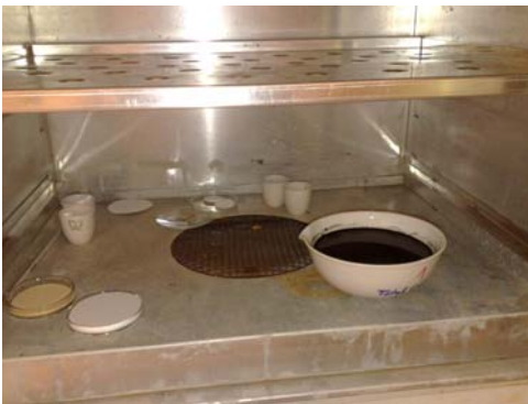
Picture Nr. 3: Bio-sludge to be evaporated for TS analysis at 105 °C
