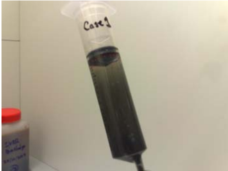
Picture Nr. 29: 1 week after installation of 4 syringes as “microsystem”. This is Case Nr. 1 (5 mL (Sleipner+15 mL of Bioreactor sample)
