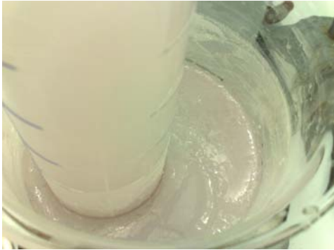
Picture Nr. 44: Precipitation of \text{CaCO}_3 due to reaction of \text{CO}_2 (present in the ambient and from bioreactor) with \text{Ca(OH)}_2
