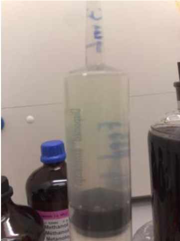
Picture Nr. 12: Feeding bioreactor with IVAR wastewater and sugar (10 g/L)
