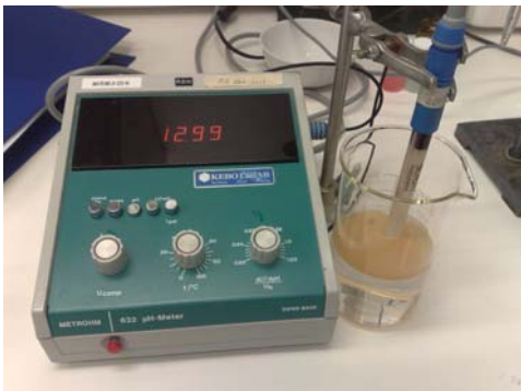
Picture Nr. 53: pH of the sample after addition of NaOH in excess
