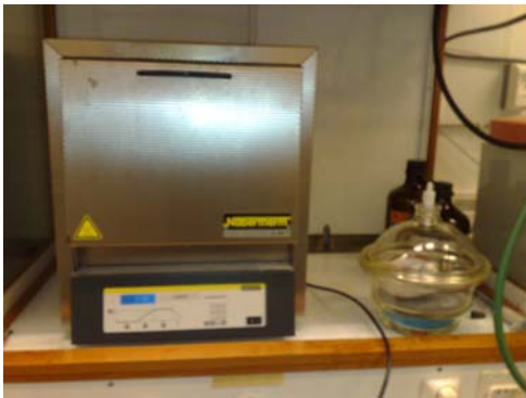
Picture Nr. 6: Bio-sludge for TVS determination (combustion at 550 °C)
