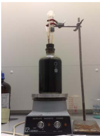
Picture Nr. 37: syringe installed to recollect gas instead of gas sampling bag
