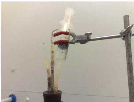
Picture Nr. 38: Gas recollected after installation of syringe (instead gas sampling bag)
