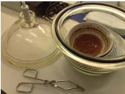
Picture Nr. 7: Bio-sludge after combustion at 550 °C
