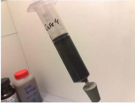
Picture Nr. 32: 1 week after installation of 4 syringes as “microsystem”. This is Case Nr. 4 (15 mL of Bioreactor sample)
