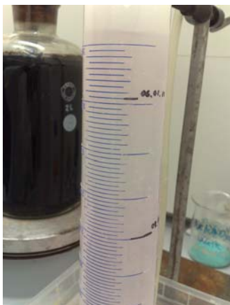
Picture Nr. 51: Gas contained in the gasometer and some bubbles are also observed along the cylinder
