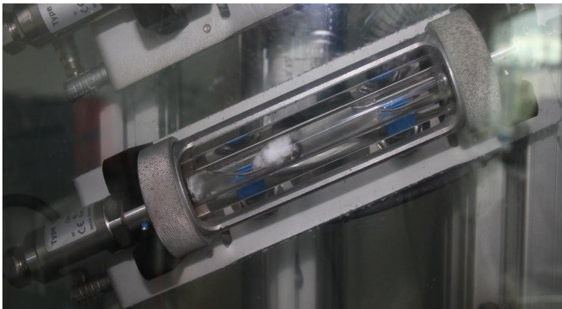
Figure 47 Formed gas hydrate in one of the tests
