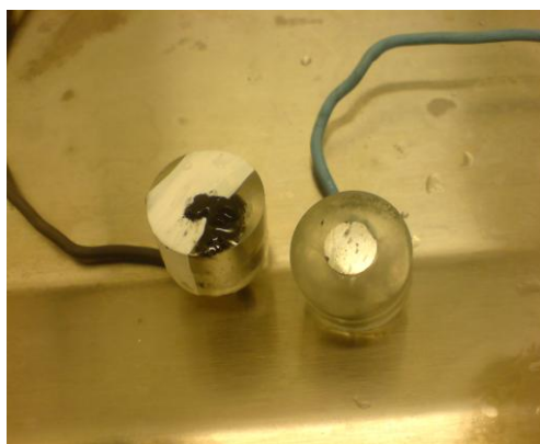
Figure 23. Picture of covered with Teflon tape and bare working electrodes.
