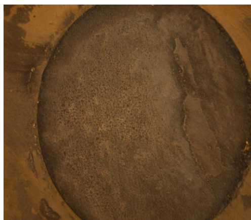
Figure 22. Surface of covered with elemental sulfur carbon steel electrode (pH10 at 80°C).
