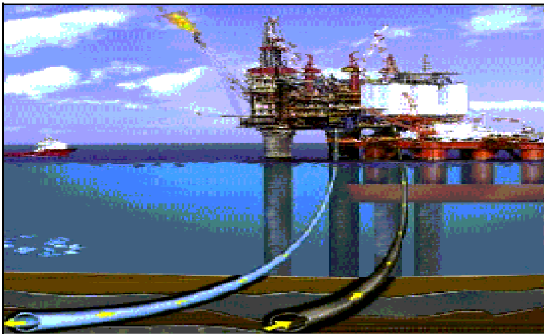
Figure1.2 Re-Injection of Separated Water From An Offshore Installation [3]
