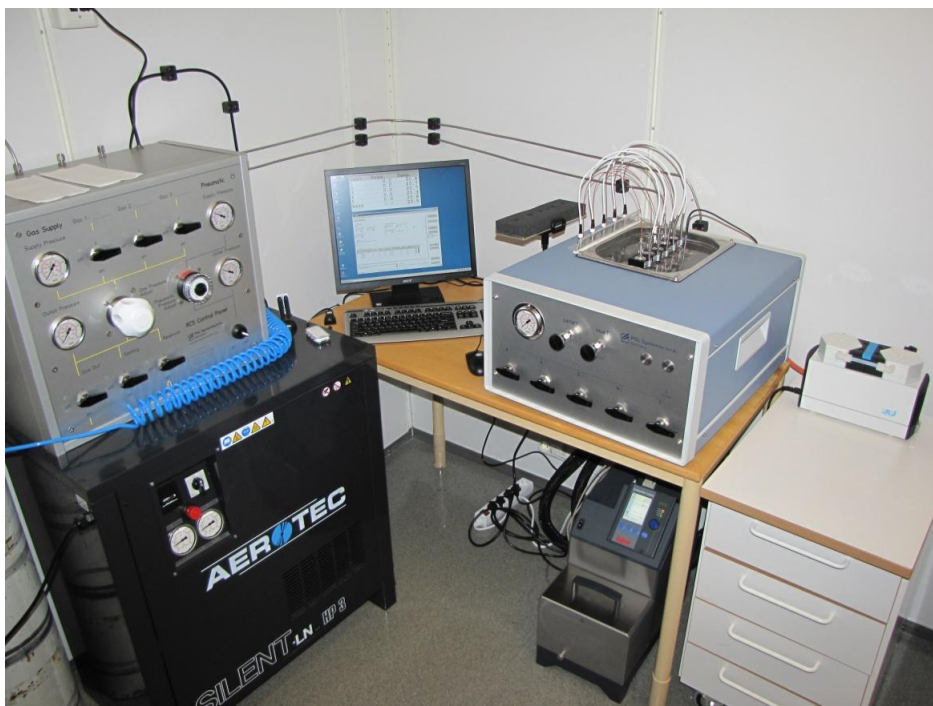
Fig. 3- 5 The complete set-up of the rig. The bottle with natural gas is barely visible in the left corner. The blue spiral pipe on top of the booster is a air gun used to dry the cells.
