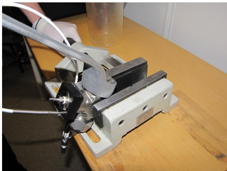
Fig. 3- 7 The cover of the cells are fastened and loosened with a big spanner.
