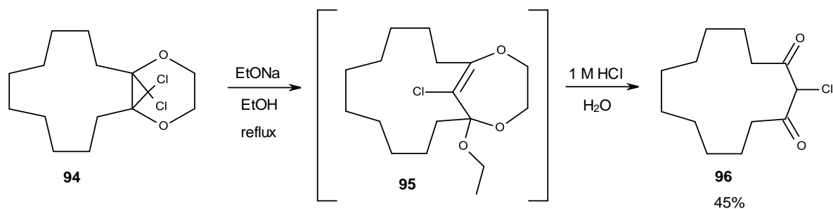
Scheme 48 Ring opening of 17,17-dichloro-13,16-dioxapropellane ( 94 ) immediately followed by acidic hydrolysis to give 2-chlorocyclotridecane-1,3-dione ( 96 ).
