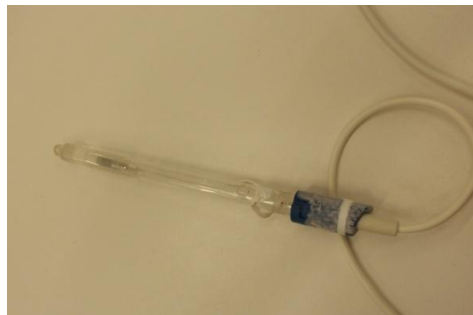
Fig. 3.4 Reference Saturated Calomel Electrode (SCE)
