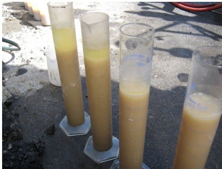
Figure 6.2 Zone sedimentation process on Run 2 samples
