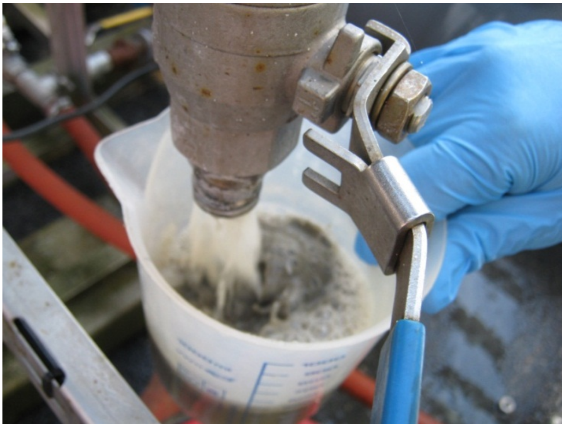
Figure 5.7 Taking water samples of treated water from the sand cyclone at SART AS
