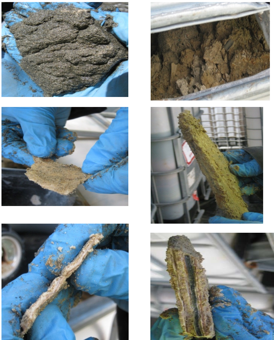
Figure 3.2 Formed calcium carbonate scale at SART AS
