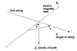
$B_0$  is the magnetic field of Earth. If this drill collar is too short, one can have additional stray magnetic fields influencing the measurements [24]. We want to consider how the pipe's field is influenced by the Earth's magnetic field. **B**<sub>0</sub>, Earth's magnetic field can be found by measurements.
