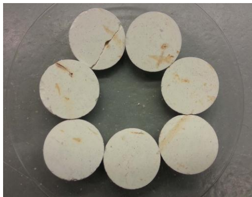
Fig. 3.24. The core which is cut in to the smaller pieces
