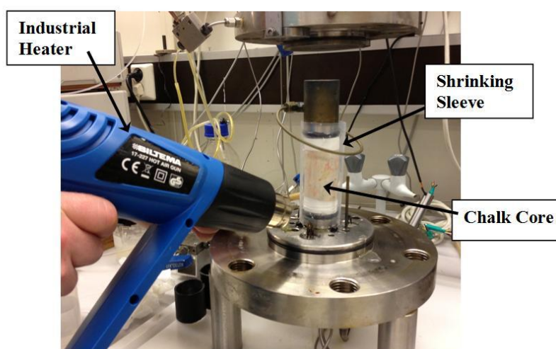
Fig. 3.19. Installing the core inside the triaxial cell
