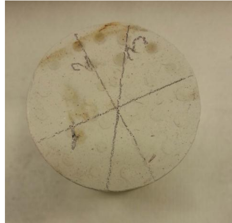
Fig. 3.20. Chalk core “KD2-LOWER” after the test, (the side view). Fig. 3.21. Chalk core “KD2-LOWER” after the test (the top view)
