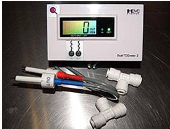
Figure 6.3: HM-Digital DM2 dual TDS monitor (image_17, 2012).
