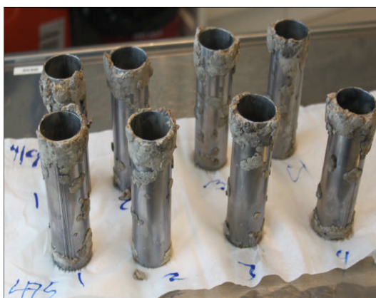
Figure 23: Clay attached to steel cylinders.
