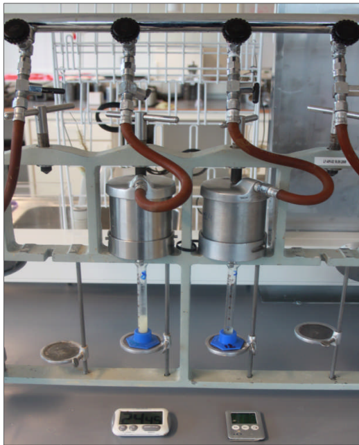
Figure 17: The API fluid loss equipment set up.
