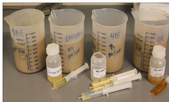
Figure 13: Mud after mixing and ready for addition of inhibitors.
