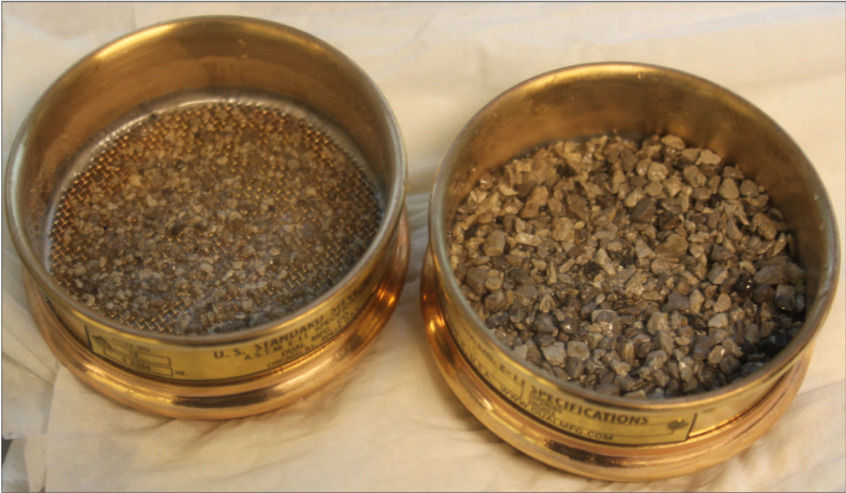
Figure 52: Dispersion result; appearance of Arne clay after the test was performed.
