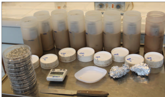
Figure 22: Mud/steel cylinder in the plastic bottles.
