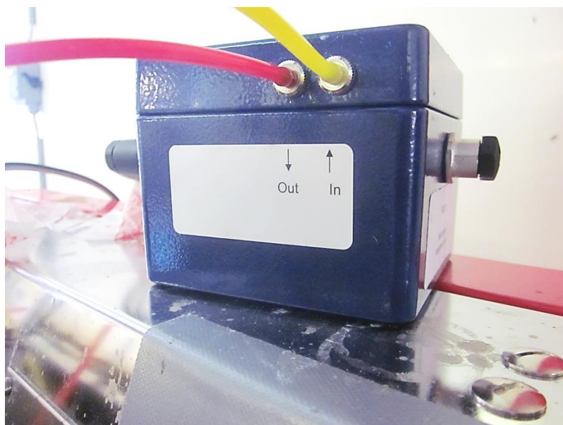
Figure 22: BlueSens Biogas sensor. Measures 0-50% CO 2 and 0-100% CH 4
