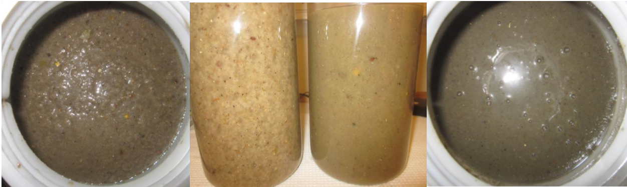
Figure 41: Raw Salsnes Sludge (left), Salsnes and Sediment Sludge (middle), Sediment Sludge (right)
