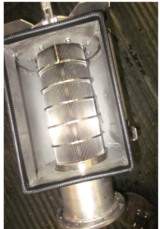
Figure 11: Dewatering unit screen that was removed for this project.
