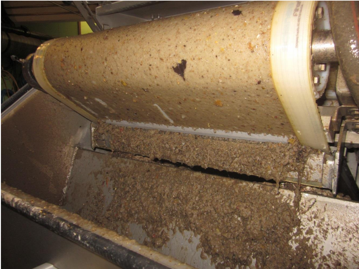
Figure 3: SF1000 used in experiment showing air knife cleaning the filter
