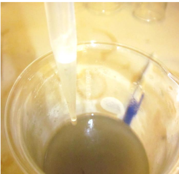
Figure 47: Sampling for COD testing, showing possible blockage of pipette.
