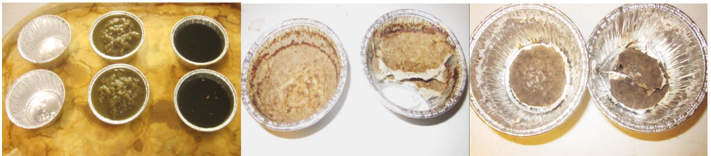
Figure 24: Wet, dried, and volatilized samples. The difference in weights determine the total and volatile solids content
