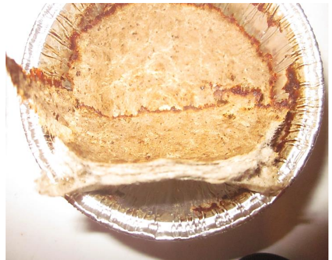
Figure 35: Salsnes sludge torn in half after drying, note the cardboard-like appearance signifying high cellulose content.
