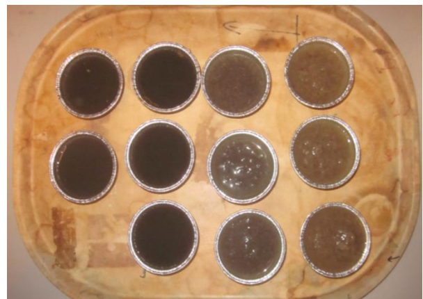
Figure 33: Wet solids in aluminum dishes prior to drying for TS/VS analysis.
