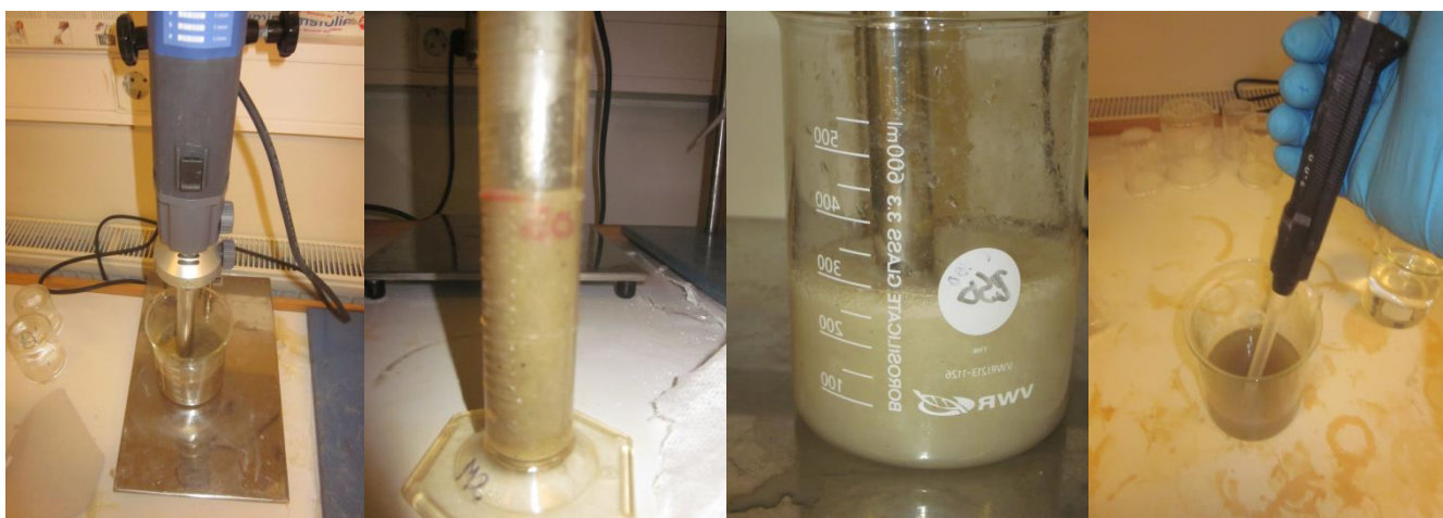
Figure 27: Emulsification with Ultra Turrax, dilute 1:10, Ultra Turrax again with diluted sample, pipet into test cuvettes.
