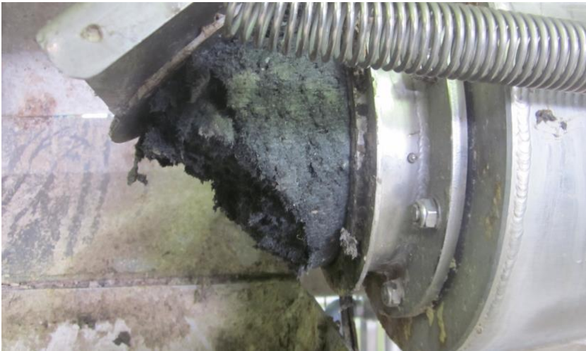
Figure 12: Dewatered sludge from SF6000 in Bangsund, Norway. Solids content ranges from 25-40%. The black color is not due to wastewater but from a charcoal addition experiment to see if dewatering was affected – typical solids look are brown or gray and lighter in color.
