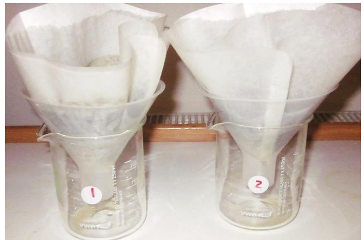
Figure 25: Filtering of digestate for alkalinity and volatile acid testing.
