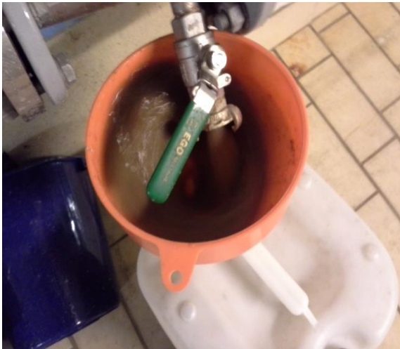
Figure 30: Sedimentation basin sludge collected ~1.2% solids
