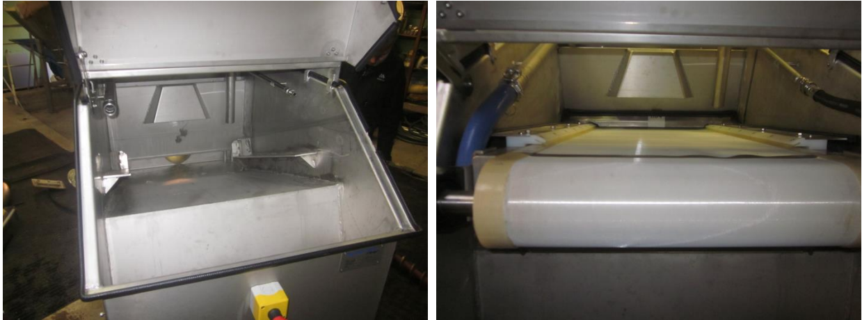
Figure 910: Salsnes filter with and without filter in place.
