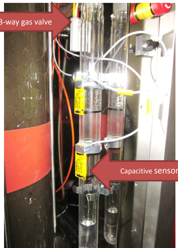
Figure 21: close up of gas clock, capacitive sensors and 3-way valve for gas flow.
