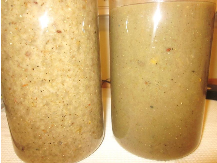
Figure 7: Salsnes Filter sludge (left) and Sedimentation sludge (right) after dilution to normalize VS%. Note the difference in consistency.
