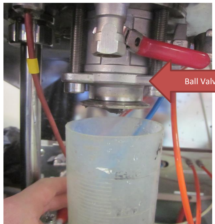
Figure 39: Digester outlet for removing solids. When onopened, fluid flows into cylinder and creates vacuum in funnel completing feed.
