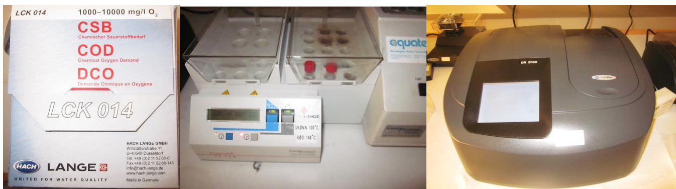
Figure 26: Hach-Lange LCK014 COD test kits, COD incubator, Hach-Lange spectrophotometer.
