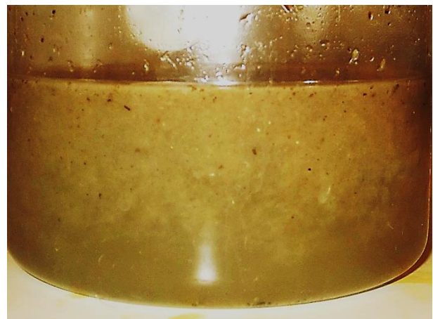
Figure 46: 1:10 Diluted Salsnes feedstock for COD analysis with large particles even after emulsification.
