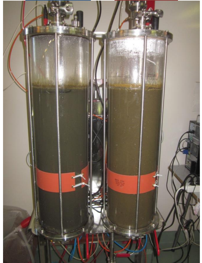
Figure 17: Dolly digester system
