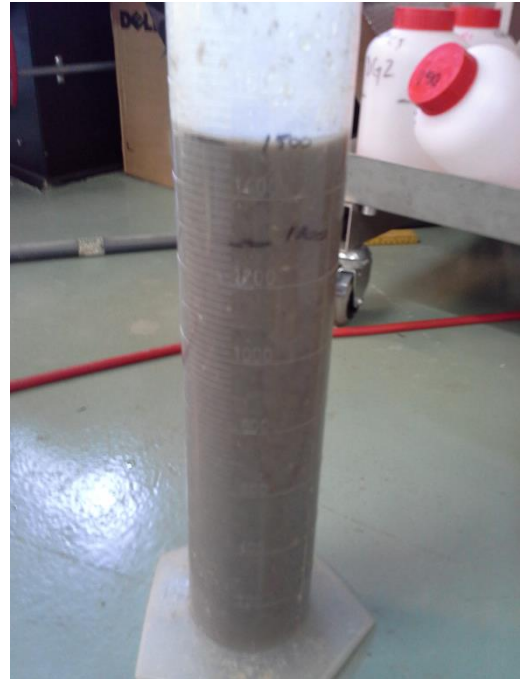
Figure 36: Measurement of sludge into graduated cylinder (1.5L/day in part 1)
