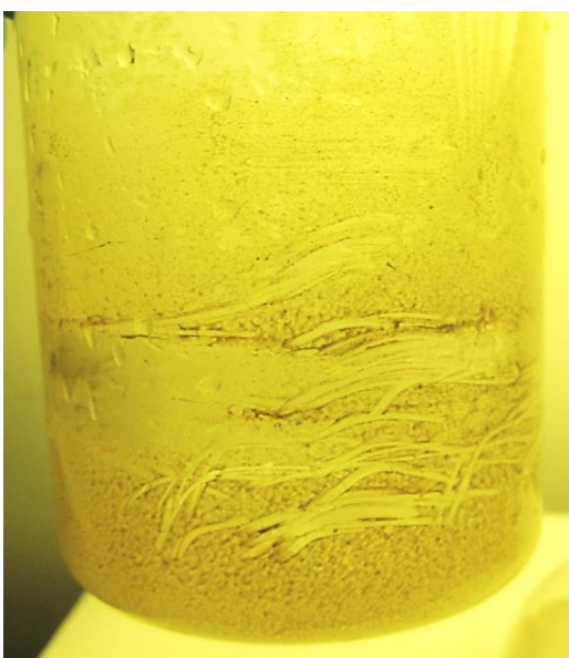
Figure 49: Empty beaker covered in fat residue after emulsification of sieve sludge.
