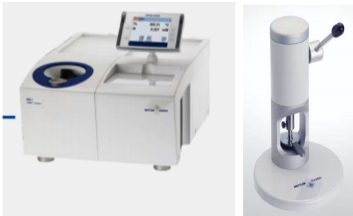
Figure 9. The figure shows a picture of the DSC machine (right side) and the crucible sealing press (left side).
