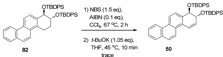
Scheme 31: Bromination and dehydrobromination of compound 82
