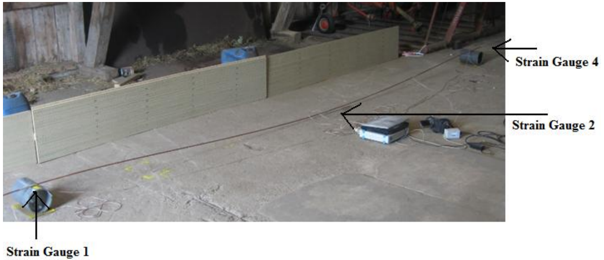
Figure 55. The placement of the strain gauges on the part of the pipeline laying on the seabed.
