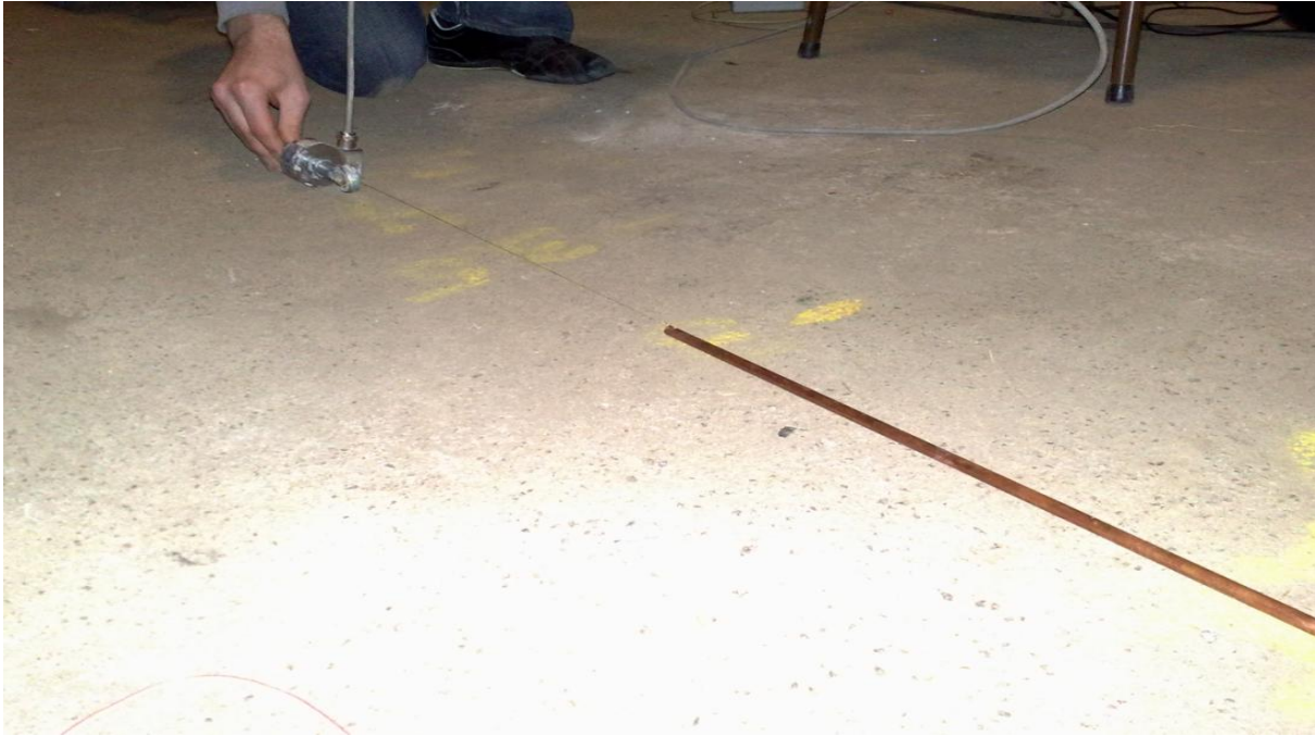
Figure 18. Measuring of the friction force on the seabed.
