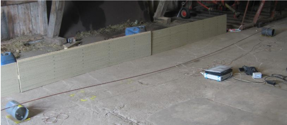
Figure 14. A free span was created by placing two obstacles on the seabed
