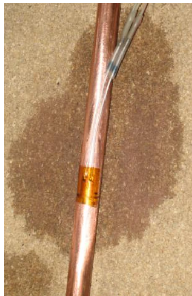
Figure 19. Strain gauge mounted on the pipeline
