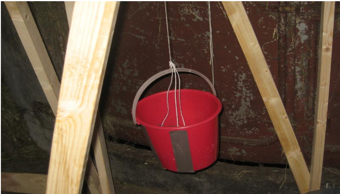
Figure 15b. The bucket that was attached to the wire. Calibrated weights were placed in the bucket.
