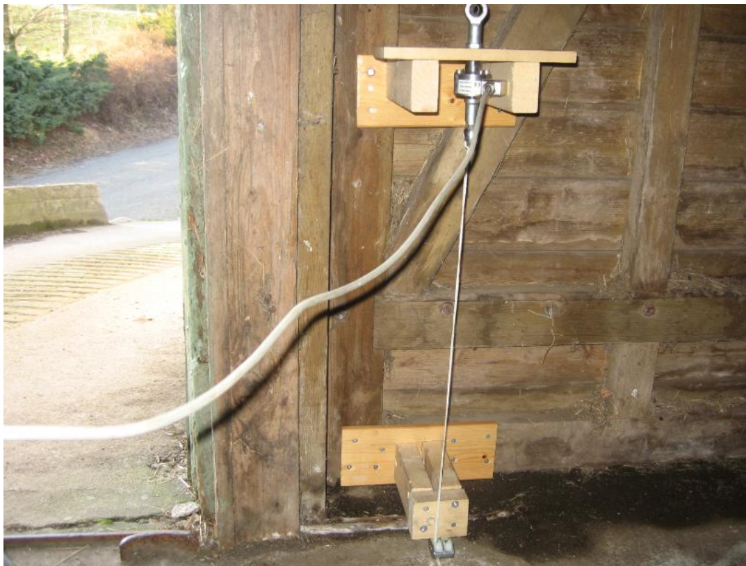
Figure 16. The load cell measuring the horizontal tension force at the end of the pipeline on the seabed
