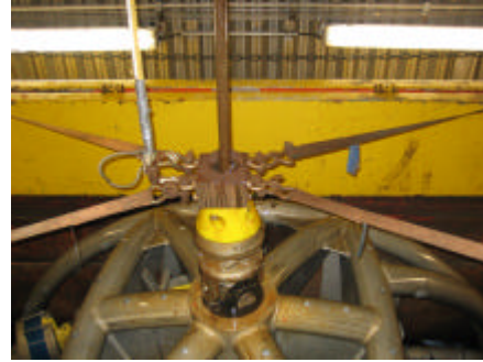
Figure 16. ROV launch/recovery with ropes and hooks through moon pool
