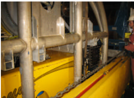
Figure 17. ROV is launching through a tight moon pool. Chains are used to guide the ROV manually through the moon pool
