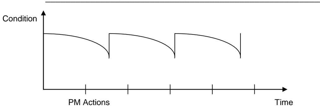
Figure 2-6. Predetermined Maintenance
