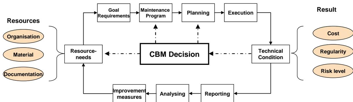
Figure 6-1. Modified maintenance management process (Based on figure 1-1, NPD, 1998)
