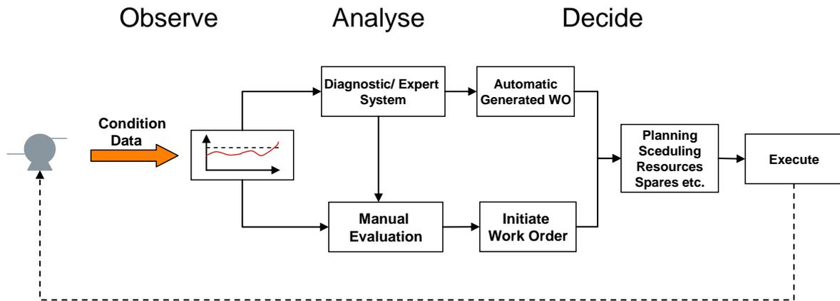
Figure 2-7. Condition Based Maintenance work process (Aker Solutions, 2009)
