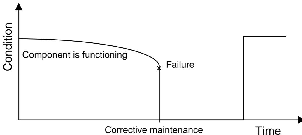
Figure 2-5. Corrective Maintenance
