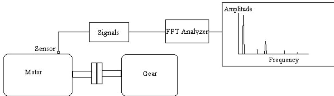
**Figure 2-8. Vibration Monitoring**
