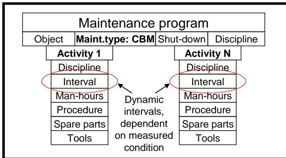
Figure 5-6. Maintenance program with CBM (Based on figure 2-4, Aker Solutions, 2010b)
