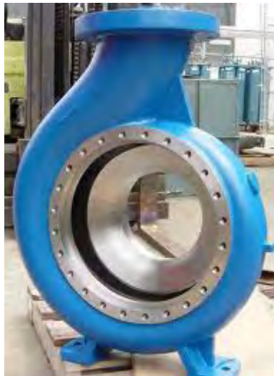
Figure 3.5: Volute casing. The cross section area is gradually expanding towards the outlet.
