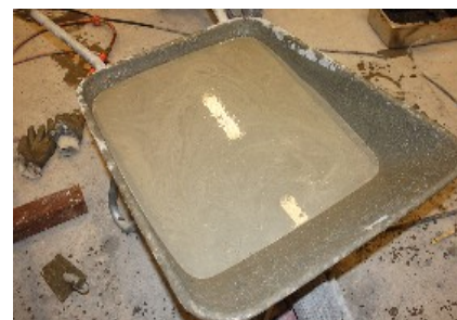
Figure 1-2: overdosing of superplasticizers admixture
