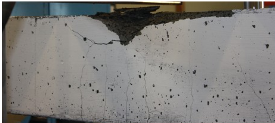
Figure 4-36: Brittle flexural failure LWC_UF
