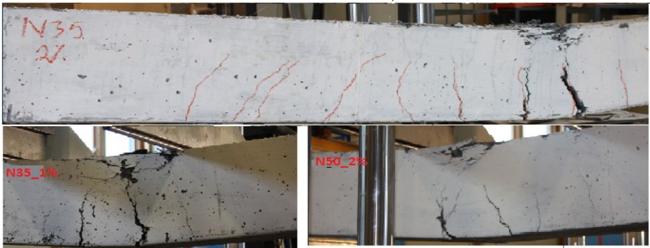
Figure 4-49: Flexural failure in beam LWC_N50_2%
