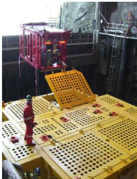
Figure 2.22: Testing of FDS hatches in dry dock
