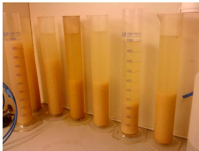
Figure 36: Settling of the sludge
