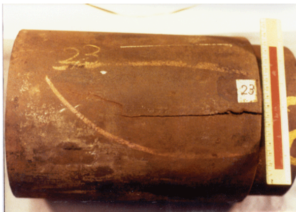
Figure 6.11: HIC in a high stress pipe (source: http://octane.nmt.edu/waterquality/corrosion/H2S.htm )
