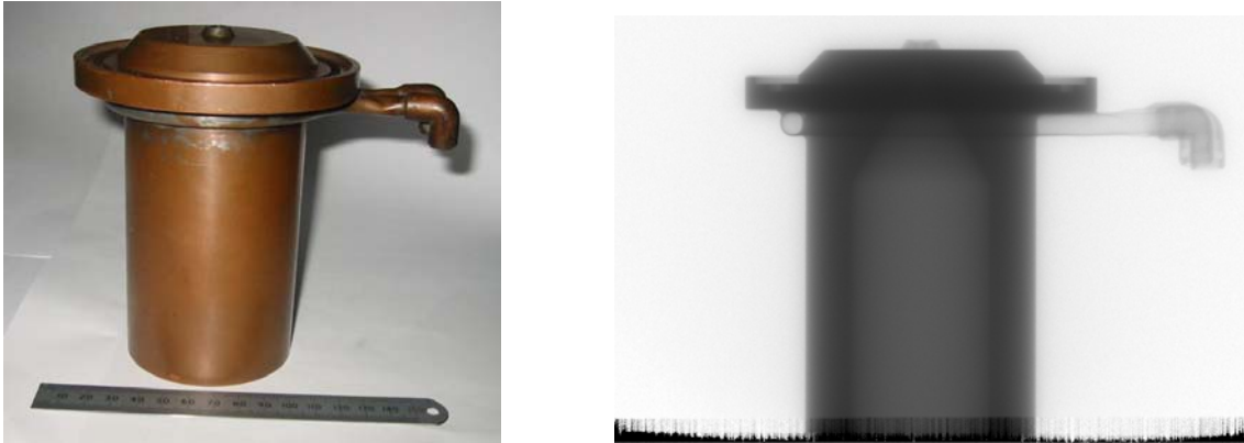
Figure 2. 18: the picture gained from a copper vessel by using digital radiography
