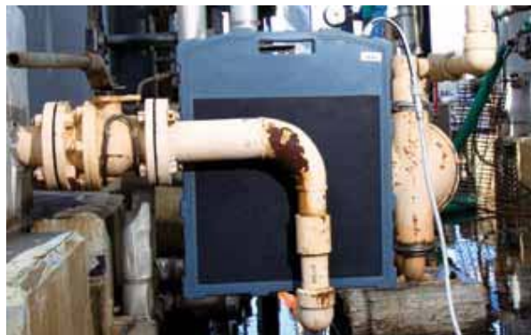
Figure 2.17: Digital detector used for digital radiographic inspection of a bend (Source: ge.com)
