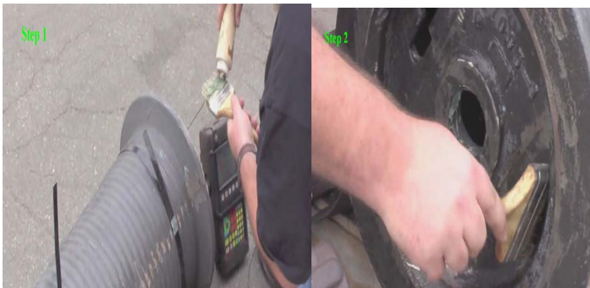
Figure 3.3: different steps of applying ultrasonic gel (couplant) to the surface of the item [Source: iqs-nde.com]
