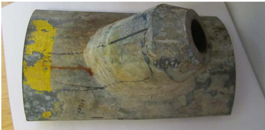
Figure 2.7: the effect of welding and turbulence leading to a leakage
