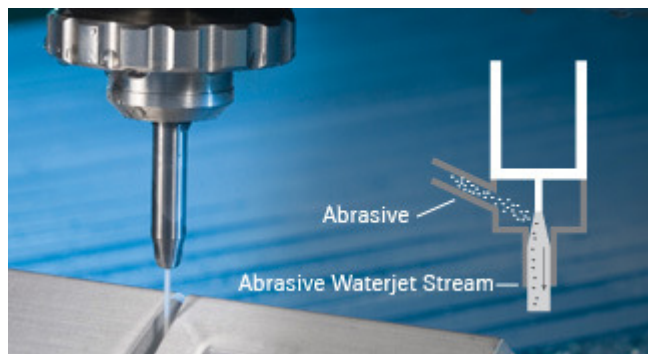
Figure 1.01 Abrasive water jet [F1]
