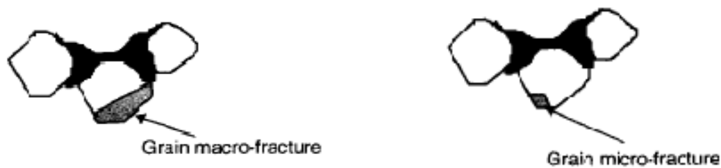
Figure 1.15 Grain fracture [F12]
