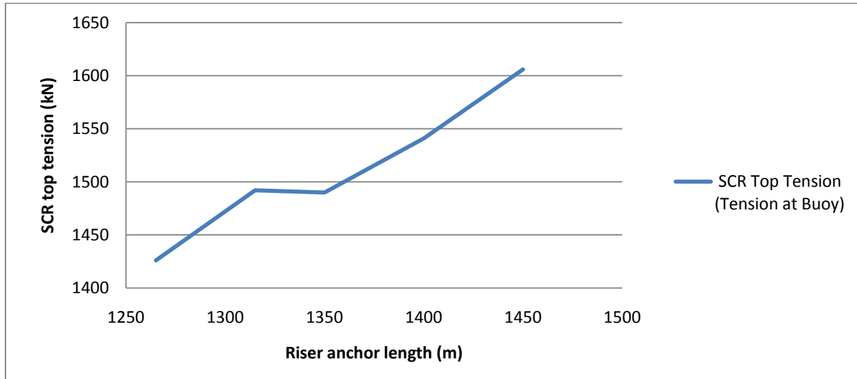
Figure 5 - 5: Sensitivity of SCR Top Tension to Riser Anchor Length, with Zero Vessel Offset and No Current – Conventional Buoy
