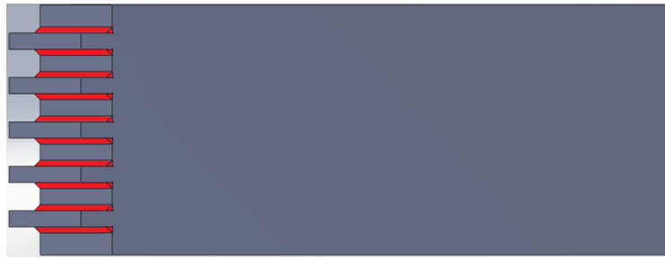
Picture 64: Full penetration K-welds on ribs in support frame
