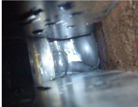
Picture 25: Extrusion of rubber through anti extrusion spring
