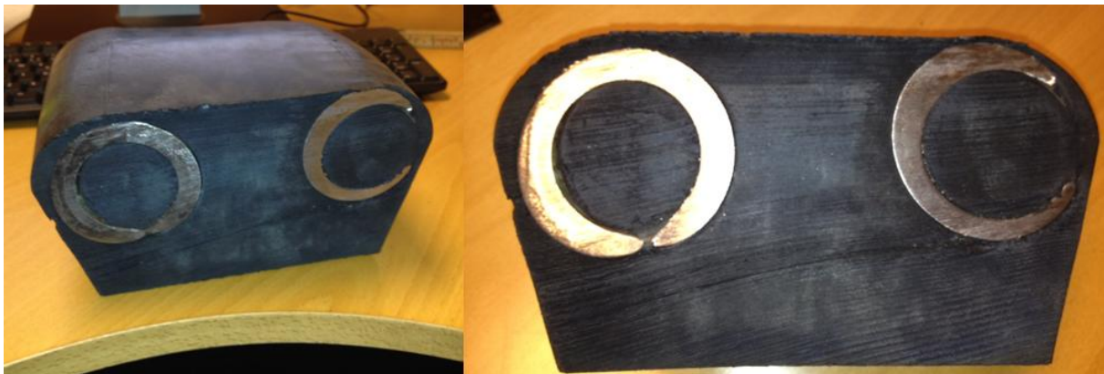
Picture 15: Cross section of packer
