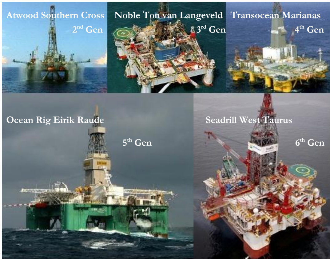
Figure 1 - Semi-Submersibles of Generations (RigLogix, 2012)
