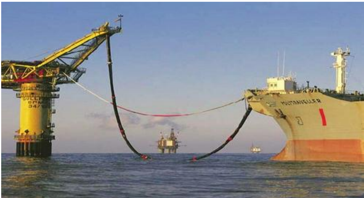
Figure 3.3: Offloading from SPM 2 to tanker [2]
