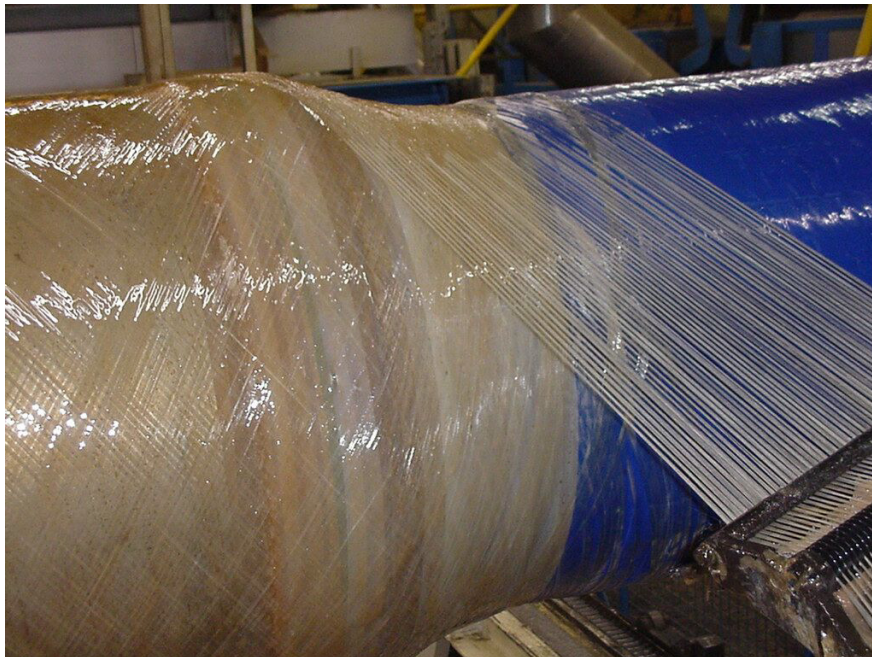
Figure 27. Manufacturing of GRE pipes.
