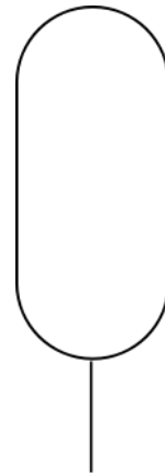
Figure 9-15 Accumulator hydraulic symbol [31]
