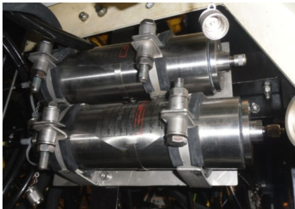
Figure 9-14 Tool shaft accumulators
