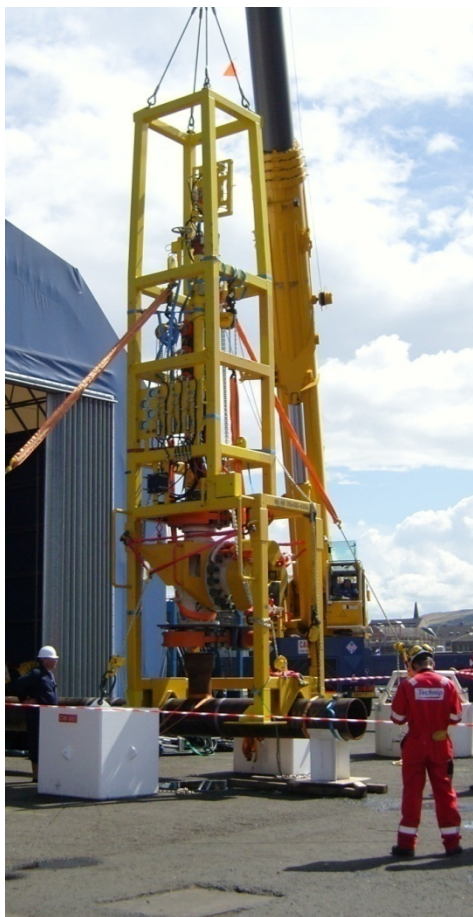
Figure 6-15 Claxton/Mirage Hot-tap cutter [11]
