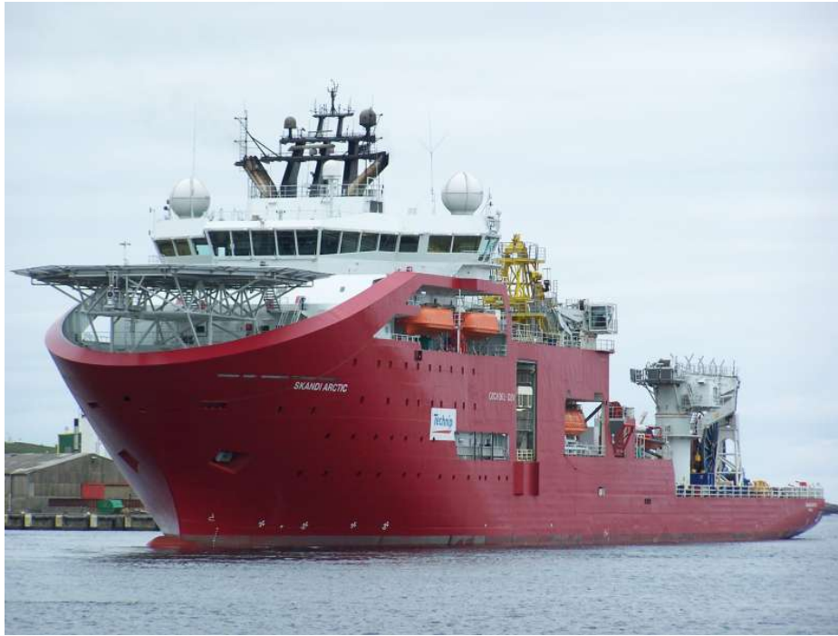
Figure 6-1 Diving support vessel, Skandi Arctic, 160 meter long [8]
