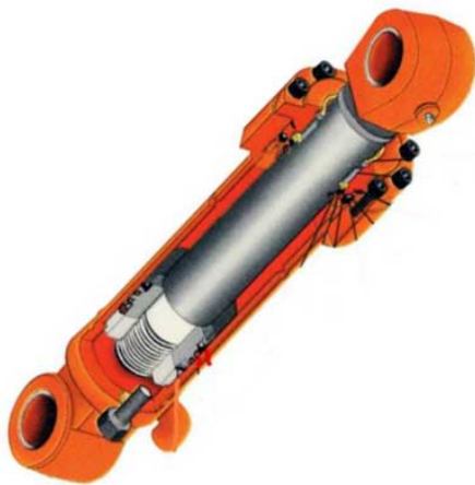
Figure 9-19 Hydraulic cylinder illustration [33]
