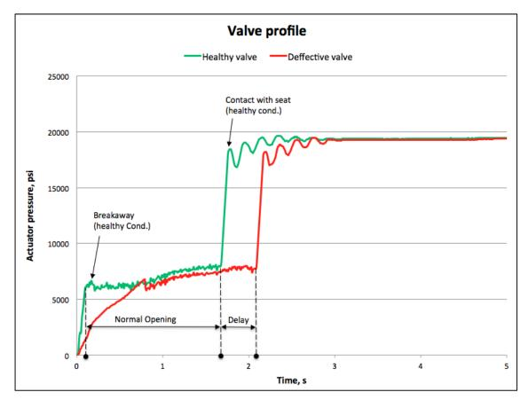
Figure 4-6 - Valve profile (opening)
