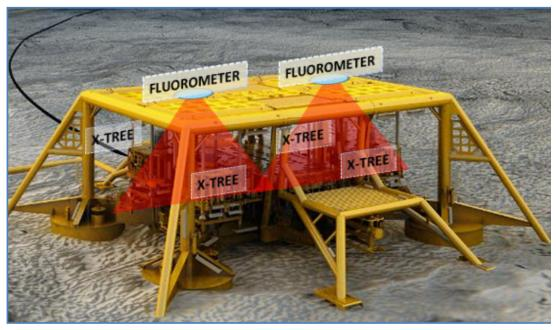
Figure 4-5- Fluorometers installed on subsea template
