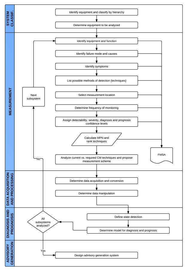
Figure 3-1 - Flowchart for implementing a condition monitoring program
