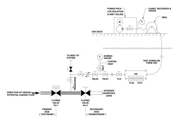
Figure 4-4 - Positive pressure test [41]
