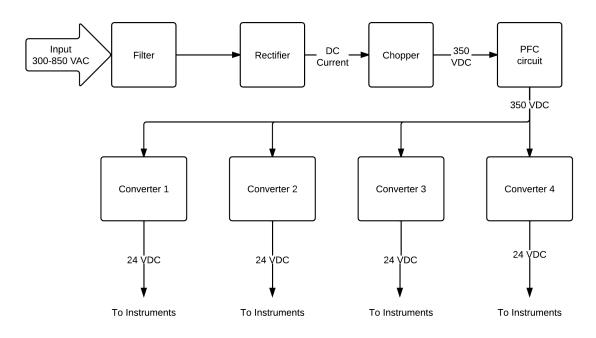
Figure 4-8 - Power supply unit flowchart
