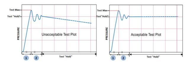
Figure 4-3 - Examples of pressure test plot [41]. 1: Pressurization, 2: Stabilization.
