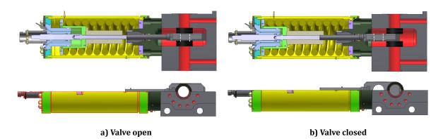
Figure 4-2 - Opening and closing of a hydraulic gate valve (source: Cameron)
