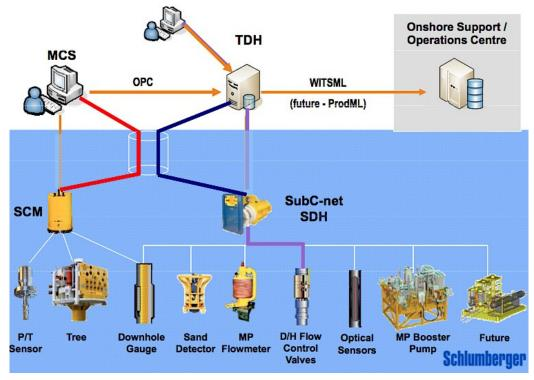
Figure 2-6 - Schlumberger parallel surveillance system [27]
