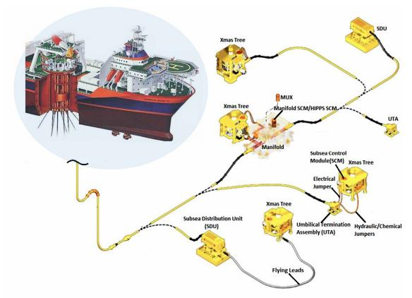
Figure 2-9 - Typical subsea production system
