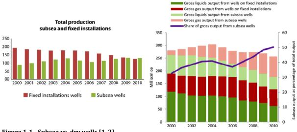
Figure 1-1 - Subsea vs. dry wells [1, 2]
