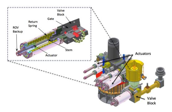
Figure 4-1 - Hydraulic valves and actuators installed on subsea XT (source: Cameron)
