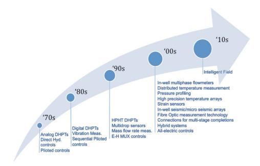
Figure 2-1 - Evolution of downhole instrumentation and subsea controls
