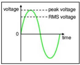
Figure 4-9 - AC peak voltage and RMS
