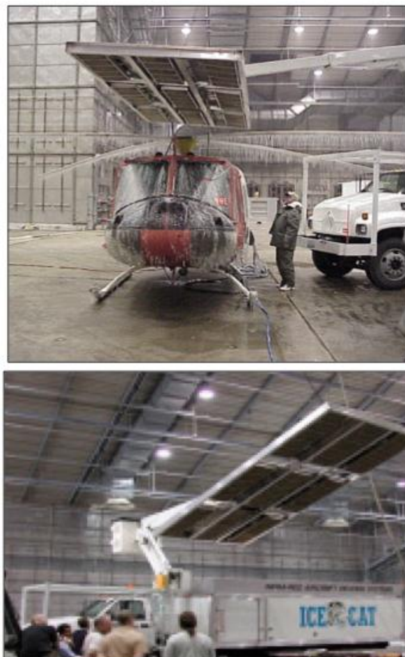
Fig. 50 Ice-Cat heater over helicopter (top) and complete Ice-Cat heater, boom, and truck system (bottom) [19]
