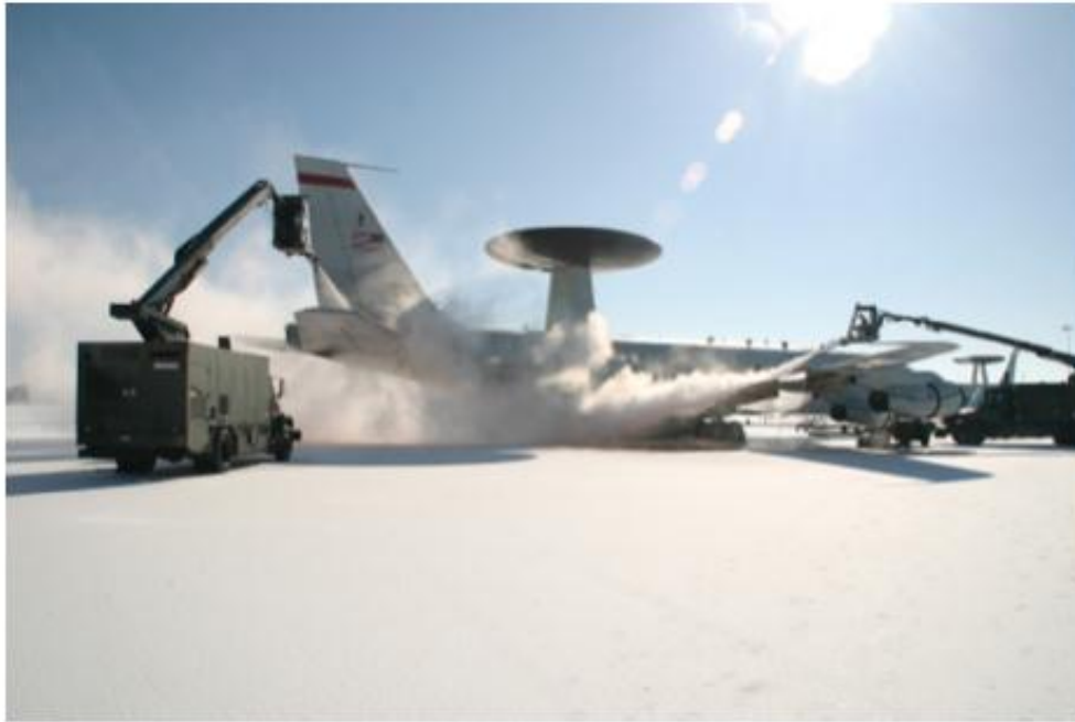
Fig. 44 De-icing of an army air-craft (Source: Air Force photo/1st Lt. Kinder Blacke)
