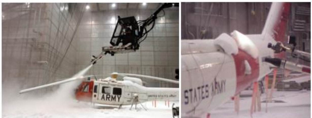
Fig. 49 AirPlus! sprays air and deicing fluid mist on helicopter blades (left). Large pieces of 10-cm-thick snow are removed from fuselage by air alone (right) [19]
