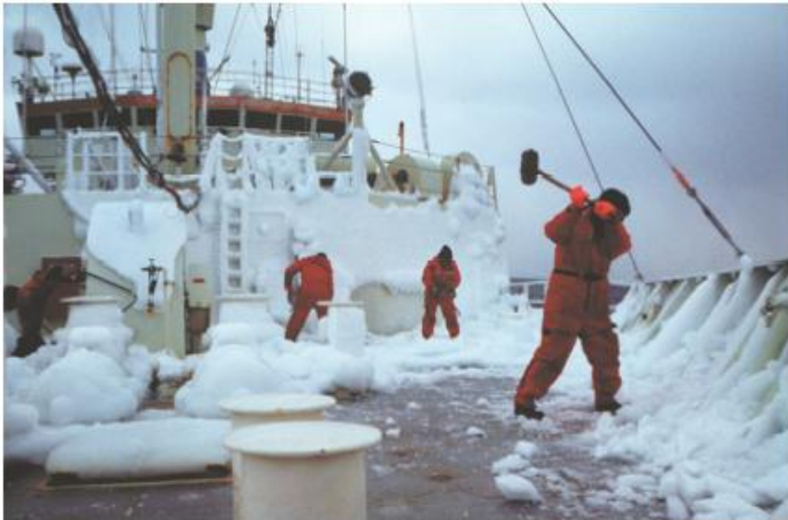
Fig. 51 Manual de-icing during a research cruise in February 1997 to the Labrador Sea
