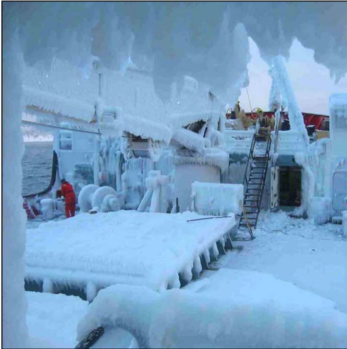
Figure 10: Icing on a vessel (Gudmestad, 2012)
