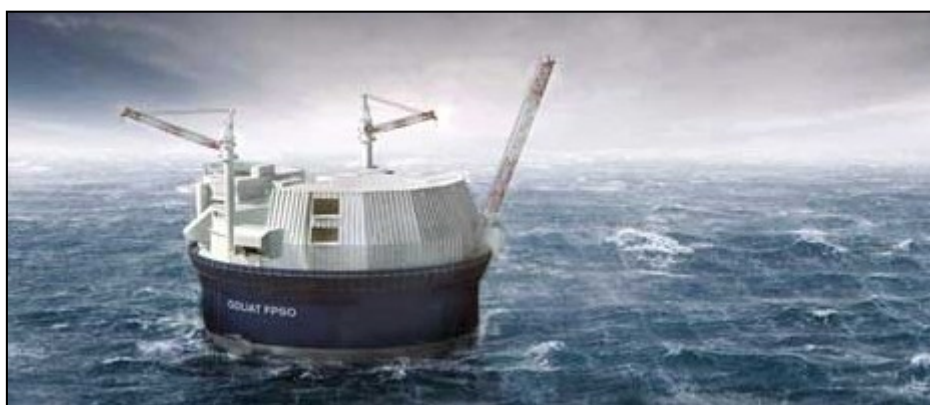
Figure 32: Goliat with cantilevered flare (APTOMAR AS, 2012)
